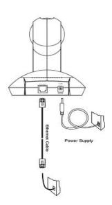
Please verify that your product package contains all the accessories listed in the foregoing Package Contents. Depending on the user's application, an Ethernet cable may be needed. The Ethernet cable should meet the specs of UTP Category 5 and not exceed 100 meters in length.
